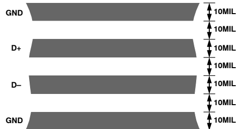
Figure 19. Arrangement of Signal Tracks
